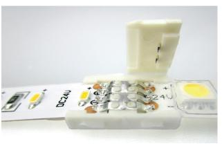
**Hint:** In certain LED Flex strips, the first LED chip is very close to the contact point. To ensure a correct and safe connecti on, the cap on one side of the clip connector must be removed. The removed cap is shown to the left of the picture. For encapsulated LED Flex strips, remove the casting first with a sharp knife. Otherwise, contacts cannot be connected. The removed casting is shown to the right of the picture.
