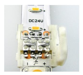
**Trick:** Install the LED Flex strip pins far apart and use a fourpin clip connector, where we will solder two contacts together (see picture). Thus, clip connectors allow the safe connection of LED Flex strips under any circumstances.
