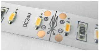
Fig 2. Scissors Icon- intended separation point of the Flex strip
