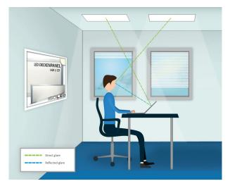
Indirect lighting, matt fixtures with low light reflection, workspace division adapted to light sources, and the elimination of specular surfaces avoid burdensome reflected glare. Thus, concentration is maintained for longer periods, which leads to higher productivity.
