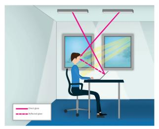
Direct glare arising from non-glare-free lighting and unobstructed sunlight strain vision and lead to fatigue. As a result, concentration lapses and the risk of making mistakes Increase. For physical work, this leads to increased risk of accidents. For this reason, we must use lights with appropriate glare ratio, install sunshades on windows, and redesign the workspace arrangement appropriately.
