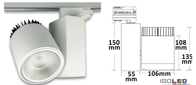
112742 | 3-PH track spotlight Fresh Meat Light, 40W, 30°-50°, white matt, with special colour temperature for meat and sausage products with dominant wavelength of 595nm
